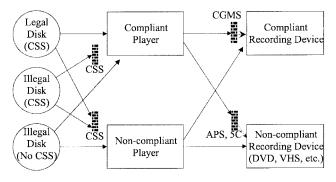
Fig. 1. DVD copy-protection system without watermarking.
