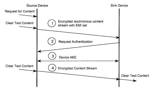
Fig. 3. Operation of 5C DTCP.
