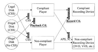
Fig. 2. DVD copy-protection system with watermarking.
