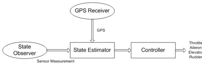
Fig. 4. Functional Structure of UAV Autopilot System.
