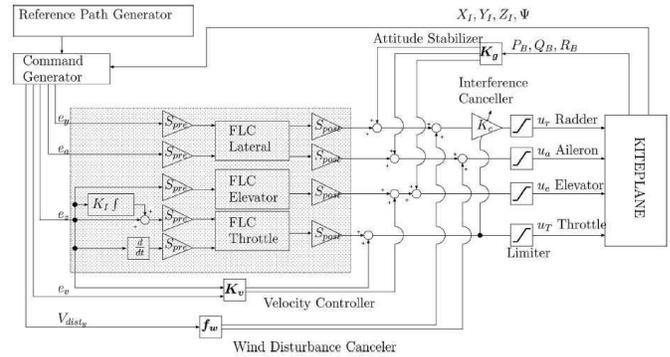
Fig. 12. FL-based Autopilot System for Kite UAV [25]
