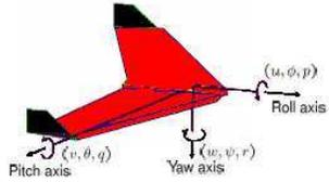
Fig. 2. Definition of UAV Axes.
