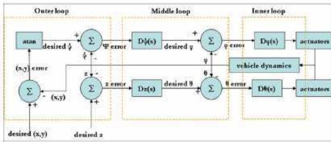
Fig. 7. PID-based Autopilot System by Crossbow [19].
