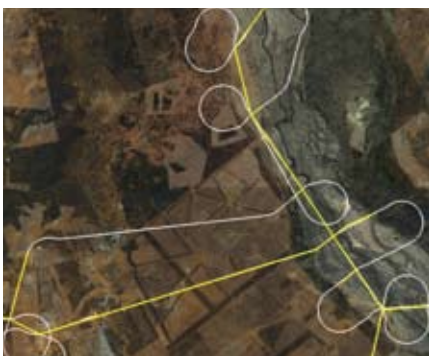
ARCAA automated flight over powerlines. White indicates flight path. Yellow indicates powerlines.
