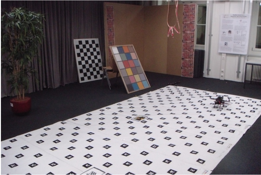
Fig. 4 Flight environment with the ARToolkit markerboard on the floor
