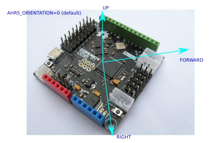
By changing the AHRS\_ORIENTATION configuration using Mission Planner or MAVproxy, you can install the Flymaple in your vehicle with other orientations. I set mine to AHRS\_ORIENTATION=1 (Yaw45) which produces this orientation:
