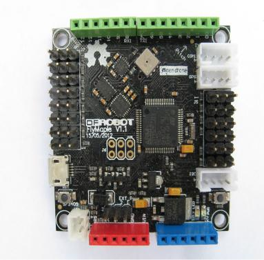
It contains a 75MHz ARM Cortex-M3 processor, 64kB SRAM, 512kBFLASH ROM, 3-axis gyroscope, 3-axis accelerometer, 3-axis compass and barometer, as well as various serial, digital and analog IO ports. More information at <u>http://www.open-drone.org/flymaple</u> Adding a GPS and a radio control receiver results in a full featured, high performance, programmable autopilot suitable for a variety of vehicles.
