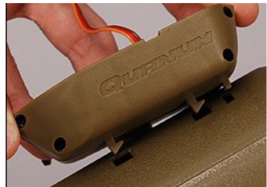
Illustration 9: The drop mechanism
