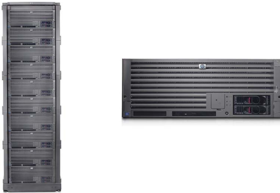
Figure 5. You can fit up to 10 rack-optimized HP Integrity rx4640 servers into a 2-meter (40U) rack.
