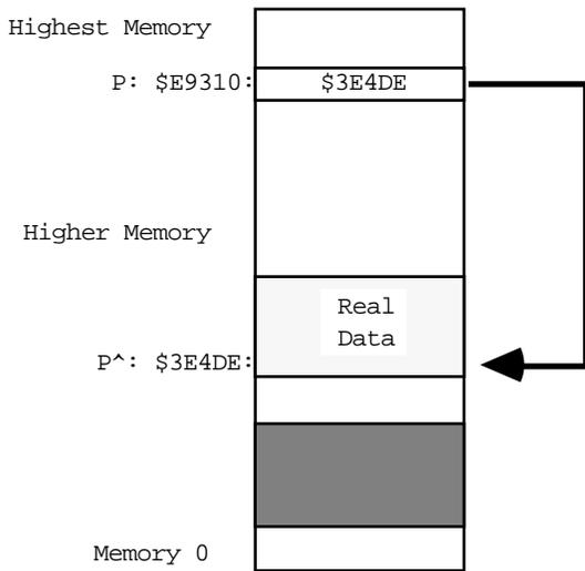
This is how a Pointer works. The address of the pointer variable itself is \$E9310 (@P) and is four bytes long. The pointer points to (contains the address of) the block at \$3E4DE (P). That memory location is where the actual data resides (P^).
