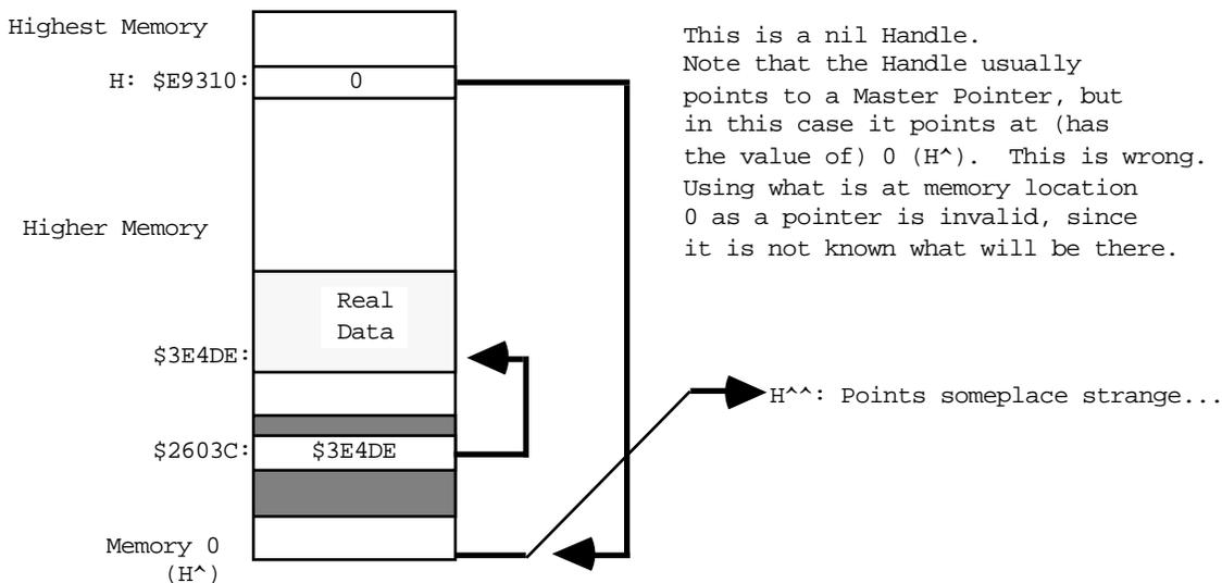
If the memory at 0 contains an odd number (numerically odd), then using it as a pointer will cause a system error with ID=2. This can be very useful, since that tells you exactly where the program is using this illegal handle, making it easy to fix. Unfortunately, there are cases where it is appropriate to pass a nil handle to ROM routines (such as GetScrap). These cases are rare, and it is **never** legal to read from or write to a nil handle.
