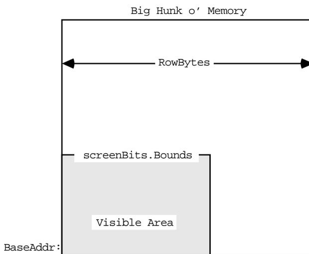
With an Ultra-Large screen, the number of bytes used for screen memory may be in the 500,000 byte range. Whenever calculations are being made to find various locations in the screen, the variables used should be able to handle larger screen sizes. For example, a 16 bit `Integer` will not be able to hold the 500,000 number, so a `LongInt` would be required. Do **not** assume that the screen size is 21,888 bytes long. `bitMaps` can be larger than 32K or 64K.
