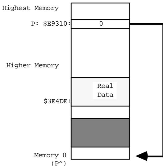
This is a nil Pointer. Note that the memory that it points to (the address) is 0 (P^). This is wrong. There is no valid data at memory location 0. Any writing to or reading from this pointer is a bug.
