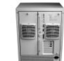
An external SCSI-1 port supports up to seven additional devices. You can add devices such as the Digital Linear Tape (DLT) drive from Quantum, which makes high-speed backups of up to 20 gigabytes per cartridge (uncompressed).
