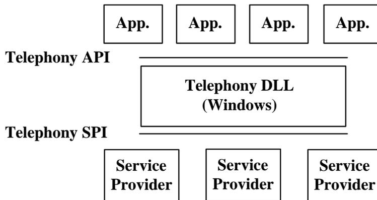
Figure 5. Windows Seamlessly Integrates Applications and Telephone Networks
