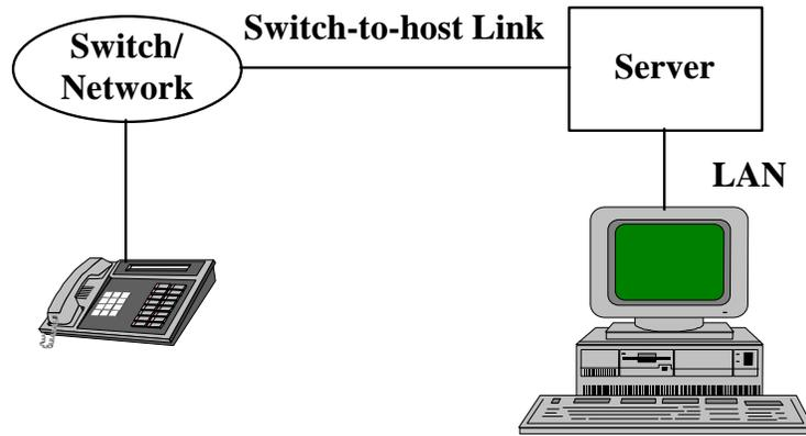
Figure 4. Connect PC via Switch-to-host Link
