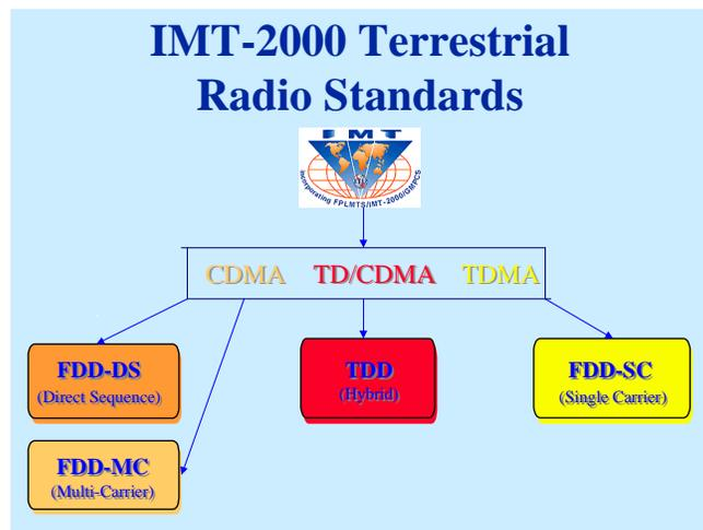
**FDD choices** include options which have been specifically optimized for evolution from **TDMA** or **CDMA** 2G systems sharing common bands as well as for deployment in new/cleared spectrum.
