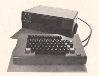
The Comter II is easily the most advanced computer terminal kit on the market. It has its own internal memory of 256 characters which combines with a highly-readable, soft orange 32 character display to provide ease of operation and information retrieval.
