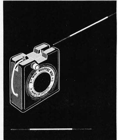
A new wire dispenser from OK Machine and Tool Company, 3455 Conner St, Bronx NY 10475, combines cutting and stripping ability in one unit. Wire is drawn out of the dispenser to the desired length, cut with the built-in plunger, and pulled through the stripping blades. Dispenser includes 50 feet (15 meters) of AWG 30 insulated solid copper wire available in four colors. People who use conventional wire wrap will find this to be an excellent addition to the tool kit. ■
