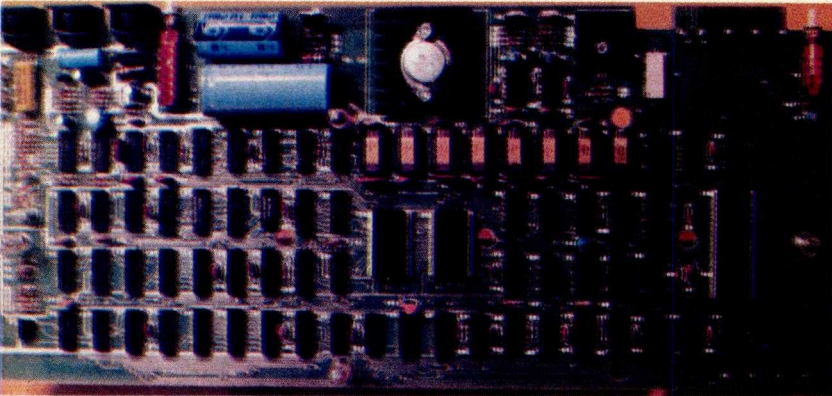
Photo 2: The single board Z-80 processor which forms the heart of the TRS-80. Note the 40 pin IO connector at upper right.
