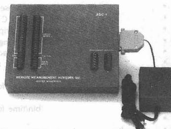
The ADC-1 serves as a real world interface for any computer or modem with a RS-232 serial port.
