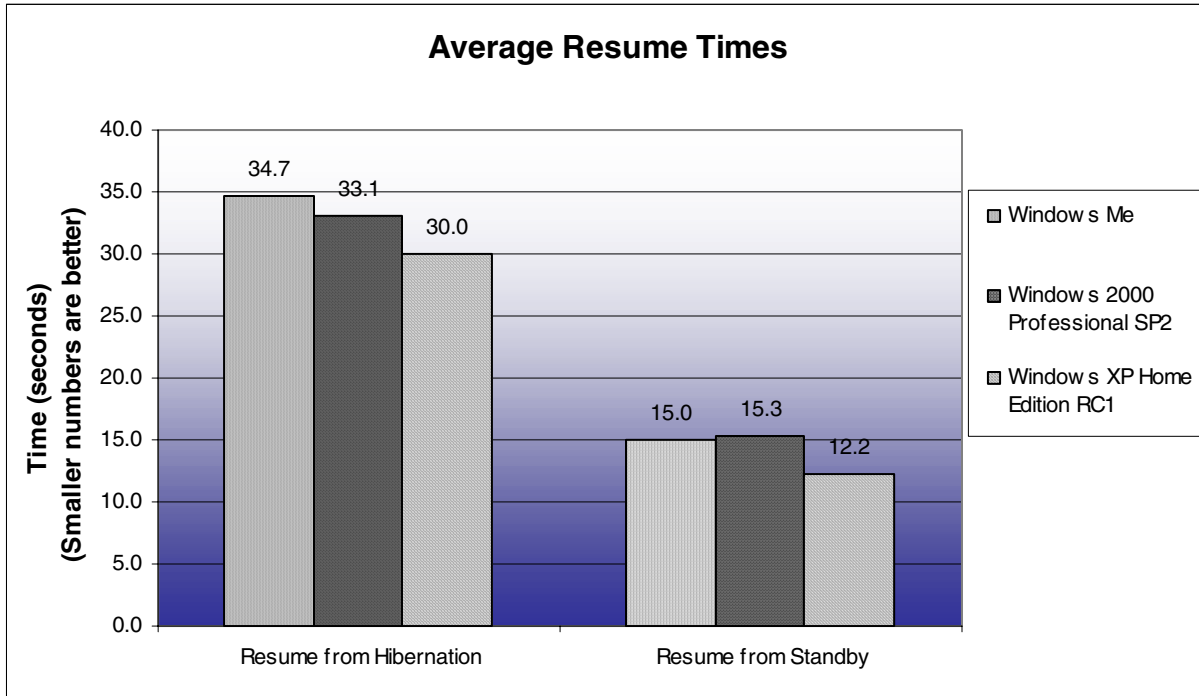
Figure 10: Average system resume performance. (Smaller numbers are better.) (Differences in the resume from standby test times would likely not be perceptible to users.)
