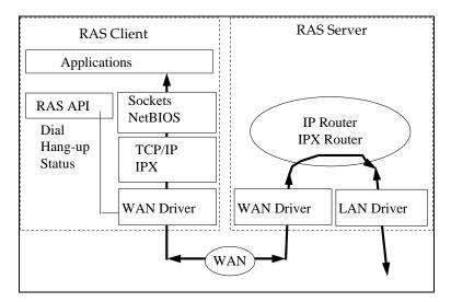
This feature significantly enhances RAS's multi-protocol support and makes it an ideal solution for NetWare and UNIX networks.
