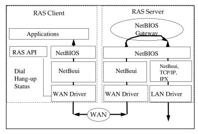
This version of Windows NT Server enhances the RAS architecture by adding IP and IPX router capability. This version of Windows NT Workstation and Windows 95 remote workstations can now run TCP/IP and IPX locally and run Windows Sockets applications or NetBIOS applications over their local TCP/IP and IPX protocols.
