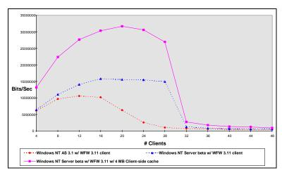
As you can see, Windows NT Server 3.51 is much faster than Windows NT Advanced Server 3.1. You can also see that using a client-side cache can result in substantially better performance. The 4-MB cache represents the recommended size for Windows for Workgroups machines that have 12-MB or more of physical memory. The combination of performance improvements and reductions in hardware pricing makes Windows NT Server even more cost-effective to deploy as a network operating system.
